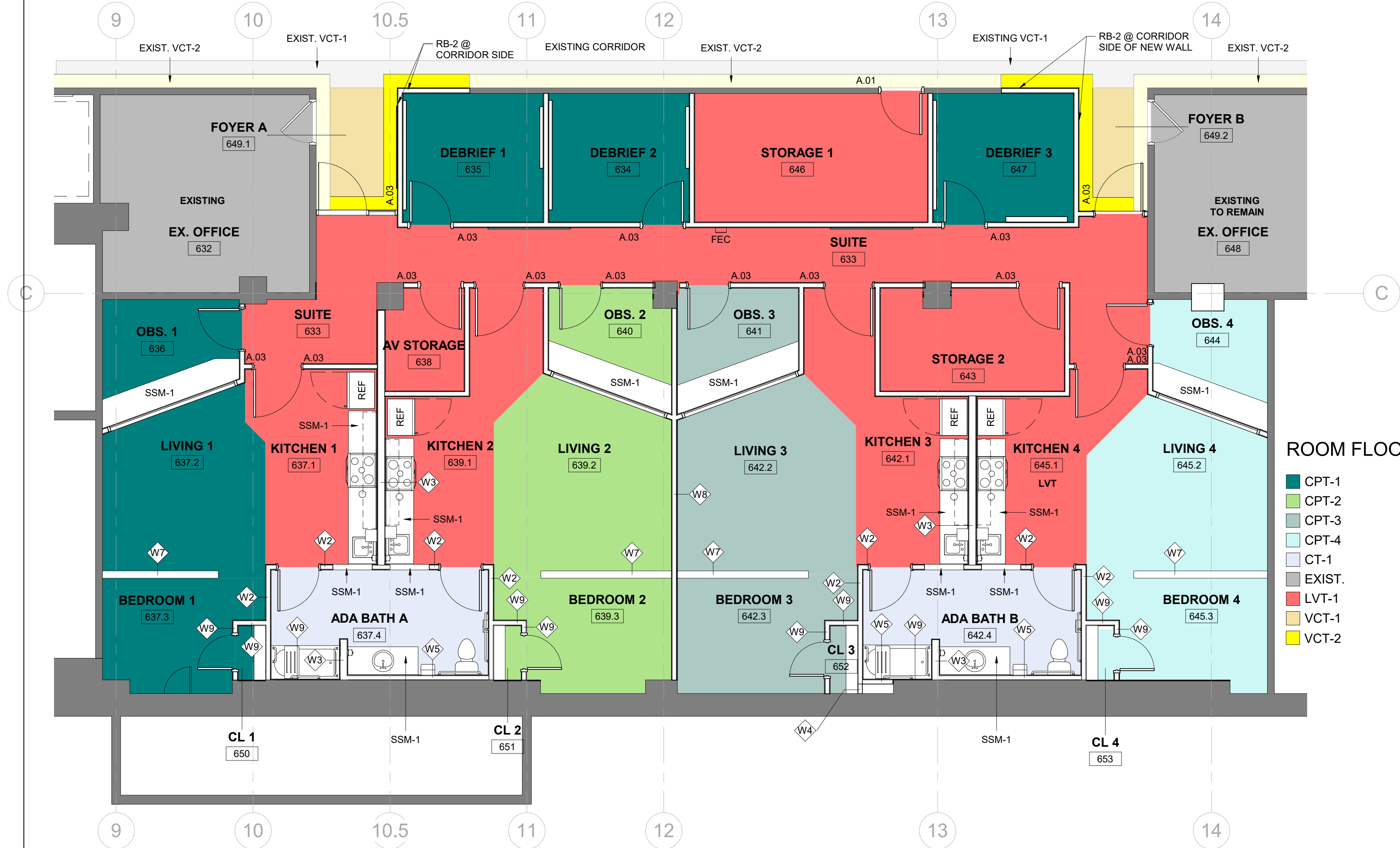
1 6TH FLOOR PARTIAL - APT. SIM. LAB FLOOR FINISH PLAN 3/16" = 1'-0"
